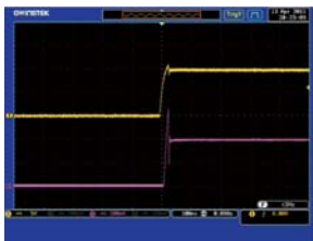
The Inrush Current and Surge Voltage occur at LED Forward Voltage ( V_f ) Under C.V Priority
