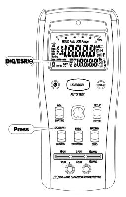
$\bullet$  Press the D/Q/ESR/ $\theta\,$  button to select the measurement function.
