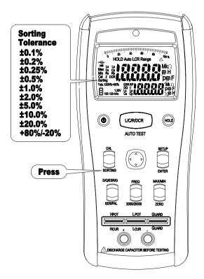
To check the accuracy of a part, press the SORTING button to enter the sorting mode. The sorting result appears on the main display, and the current value appears on the sub display.
