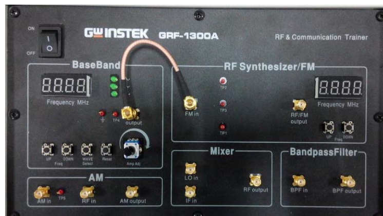
Figure A-3. Connection diagram between different modules
