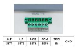
Another difference, while comparing with GDM-8251A, is that the Digital I/O of GDM-8351 provides two different modes which are general and self-definition. With the general mode, Digital I/O will output Hi Fail, Lo Fail, Pass and EOM (measurement results) based upon the results of the compare function and, furthermore, external trigger input is also provided. Under the self-definition mode, users can define output conditions for four pins (SET1~SET4) to execute the external control.
