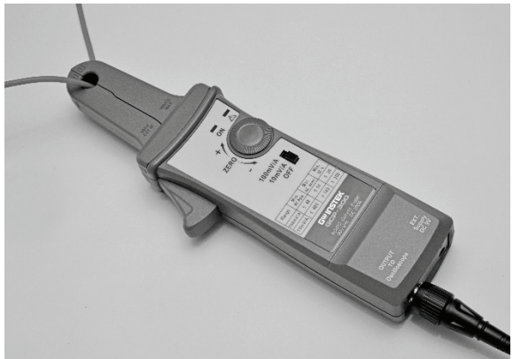
Figure 2. Connecting the GCP-300 current probe.
