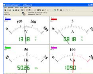
Multimeter Display for Up To 4 Channels
