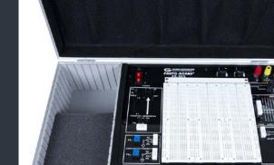
Global Specialties Model PB-503C is a Portable Analog & Digital Design Workstation. The PB-503C's newly updated, robust design makes it a trainer suitable for all levels of electronics instruction and design. With its new heavy duty case design, it has plenty of room for storage, making it highly suitable for distance learning applications and students on the go.
