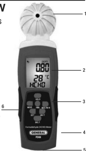
Fig. 1. The controls, indicators and physical structures of the FD08
