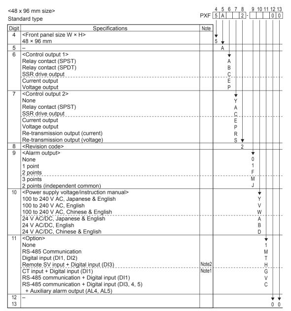
Note 1: When using the CT input as a heater burnout alarm, add one alarm output for it in the 9th code.
