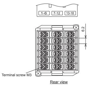
Terminal block is not attached to unused terminals (terminal 7 to 12) according to the model.
