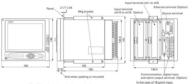
(Note) When placing the main unit on another instrument or on the floor, allow a space of 100mm or more between the unit and instrument or the floor.
