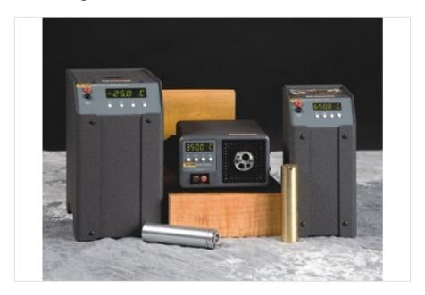
**Fluke 9103** Fluke Calibration 9103 Field Dry-Well
