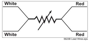
Figure 1. PRT Schematic
