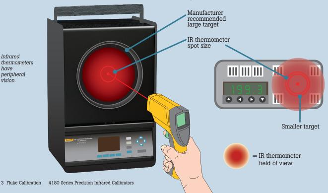
Infrared thermometers have peripheral vision.
