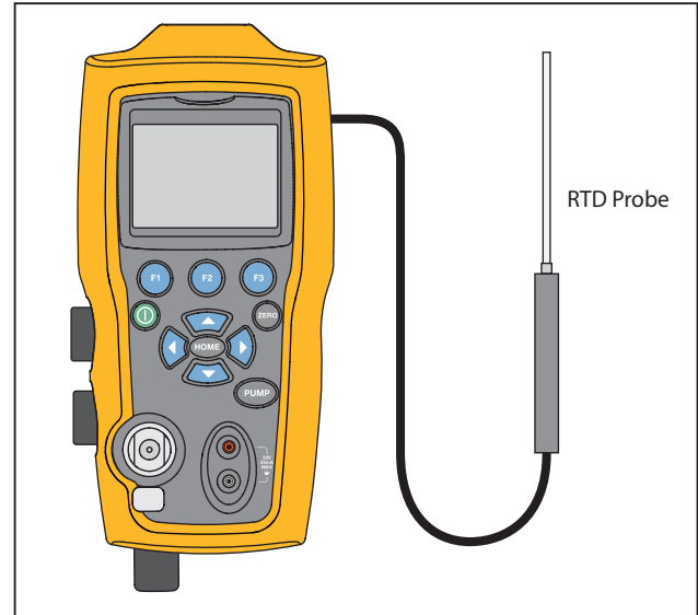
Figure 7. Temperature Measurement with RTD Probe
