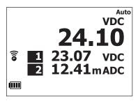
To verify which measurement in the display of the Product belongs to which test tool, look for the test tool with the same ID number on its display. Or, push to highlight a test tool in the list. The s button on the test tool blinks at a faster rate.
