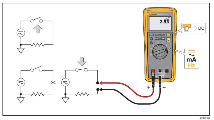
Figure 6. AC and DC Current Measurements
