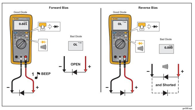
Figure 7. Diode Test
