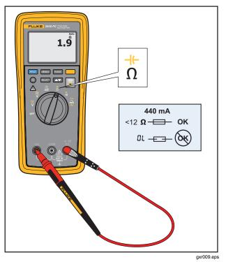
Figure 9. Fuse Test
