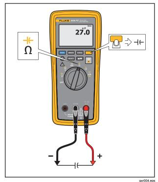
Figure 4. Capacitance Measurements
