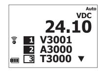
You can select up to 3 test tools and show their measurements on the Product display. The Product stays in the test tool selection mode for approximately 2 minutes.
