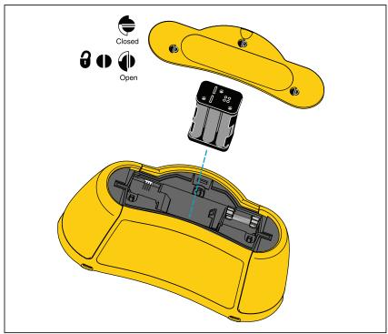
Figure 17. Battery Replacement
