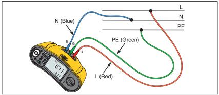
Figure 4. Connection for Safety Pretest
