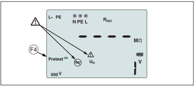
Figure 5. Display for Safety Pretest
