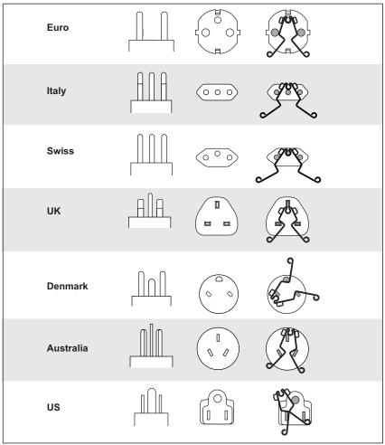
Figure 3. Country-Specific Zero Adapter Configurations
