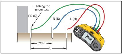
Figure 12. Earth Resistance Test Connection
