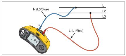
Figure 7. 3-Phase System Measurement
