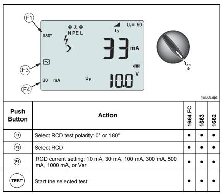
2. Press (\*) to select the RCD current rating (10, 30, 100, 300, 500, 1000 mA). If the RCD has a special nominal current setting other than the standard options, you can use a custom setting with the Var mode.
