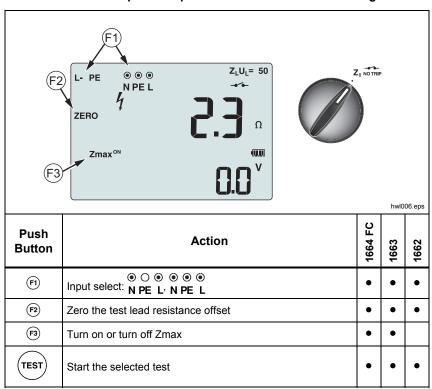
2. Press (r) to select L-PE. The display shows the  $Z_L$  and --- indicators.
