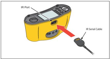
Figure 16. IR Serial Cable Attachment
