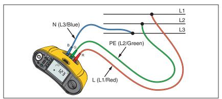
Figure 10. Phase Rotation Test Connection
