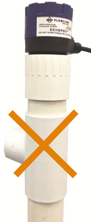
Avoid the use of a tee within the stand pipe. A tee can create false signals impeding the sensor's performance.
