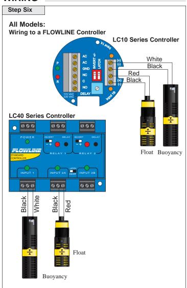
Note: Above wiring is for NO operation (open circuit when switch is dry and closed circuit when switch is wet). To wire NC (closed circuit when dry and open circuit when wet), use RED and BLACK wires for the LV10-3\_1 or reverse the float for the LV10-2\_1. Use the shield to protect the cable from electrical noise. Attach to either the Shield terminal or the ground terminal.
