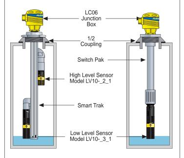
Note: Avoid installing the LV10 in magnetized metal tanks. Doing so will activate the internal reed switch.
