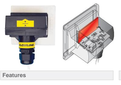
The general purpose non-intrusive capacitance level switch provides reliable liquid level detection of water based conductive liquids with non-coating and/or scaling characteristics with a 1A relay output. Media examples include hydrochloric, sulfuric acid and water. The liquid level sensor is bracket mounted on the exterior wall of non-metallic tanks and applied as a high level alarm or low level alarm.
