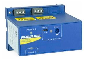
The general purpose flow controller is offered in two configurations for low-flow pump and process protection. The LC80 accepts one flow sensor input and provides one 10A relay for low flow control. The LC82 accepts two flow sensor inputs and provides two 10A relays for dual low flow control. Package this flow controller with our liquid or gas flow switch sensors. For field mount installation, add a single or dual controller NEMA box.
