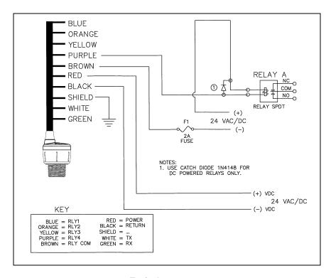
Typical Wiring Diagram
