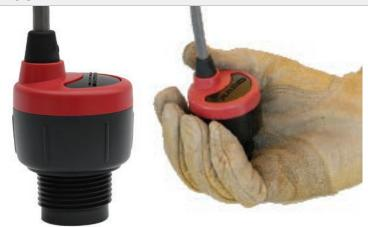
The general purpose ultrasonic level switch provides continuous level detection up to 49.2" (1.25m) with 4 programmable relays for level switch or level control functions, and is configured via our free WebCal software. The embedded level controller can lower cost by replacing external control hardware. This non-contact liquid level sensor is ideally suited for corrosive, sticky or dirty liquids, and is broadly selected for small day tank, skid, IBC, sump and process tank level applications.
