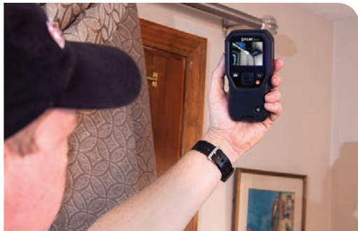
Scanning ceiling & wall joint for moisture issues
