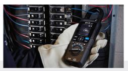
DIAGNOSE EFFICIENTLY Quickly verify problems, check loads, and validate hot spots
