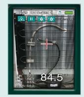
Large 2.2" color video LCD displays measurement area with temperature/humidity, min/max/avg, date,
