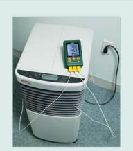
Simultaneously record and time stamp multiple temperature readings.
