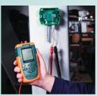
Precision "source" for calibrating process devices.
