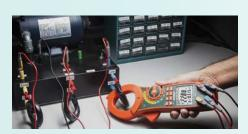
Connects to all three voltage phases simultaneously without having to move test leads from phase to phase.
