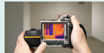
Infrared cameras quickly locate moisture related problems
