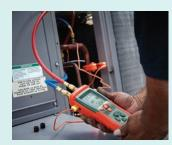
Extech's Heavy duty Digital Manifold/Pressure Gauge simultaneously measures suction line or liquid line pressure and line temperature to calculate and display superheat and sub cooling for A/C units. It also has dual inputs measuring differential pressure (P1-P2) and Type K temperature (T1-T2). For use with R22 and R410A refrigerants. Included are heavy duty connection hoses, Type K Temperature Clamp probe, and bead wire Temperature probe.
