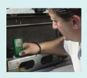
Extech's CG104 offers a quick, one-handed operation, non-destructive measurement of the thickness of ferrous and non-ferrous substrates. Its unique reversible display allows you to take readings in challenging angles of area being measured.
