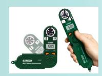
Pocket Thermo-Anemometer measures Windspeed in ft/min, MPH, m/s, km/h, Knots and Beaufort Force with 10 second averaging function. Additional measurements include: Temperature, Relative Humidity, Dew Point, Wet Bulb, and Windchill. The built-in compass provides wind direction/ 360° readings and has an easy-to-use calibration procedure for improved accuracy.
