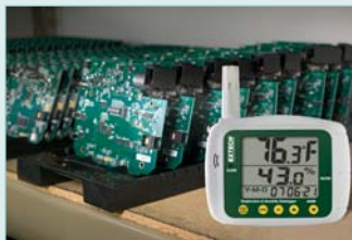
Displays and logs the Humidity and Temperature levels in Production areas
