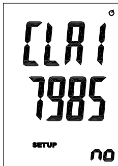
Fig. 5 Screen shows 17,985 readings left in memory.
