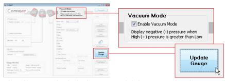
Select Enable Vacuum Mode and update the gauge to properly display a negative pressure value.
