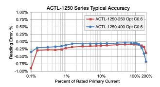
Graphs show typical performance at 23°C, 60 Hz. Graph shows a positive phase angle when the output leads the primary current.
