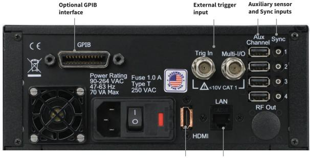
HDMI interfaceLANHDMI output for remoteLANfront panel displayether
