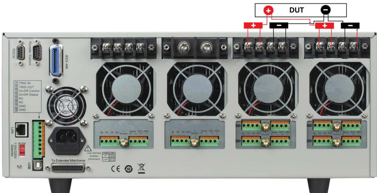
Figure 3.2 Parallel Module Connection
