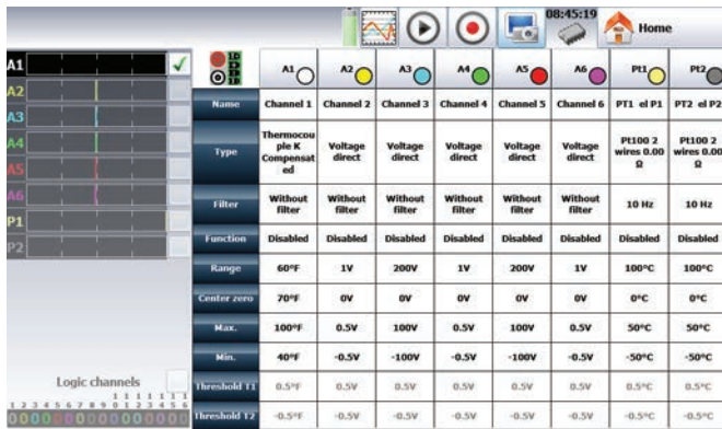
Channel setup displays all parameters on a single screen
