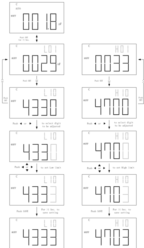
Figure 25 - Steps to Set H/Limits
