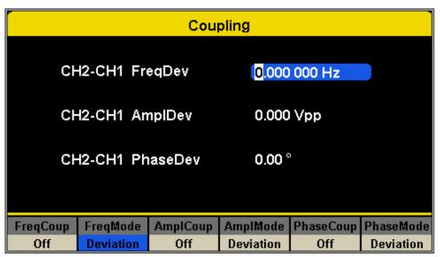
Figure 60 - Channel Coupling
