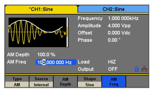
Figure 28 - Setting Interface of AM Modulation
