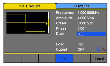
Figure 11 - Duty Cycle of a Square Waveform
