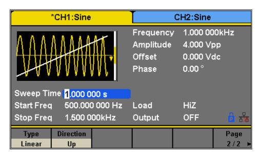
Figure 40 - Linear Sweep Interface
