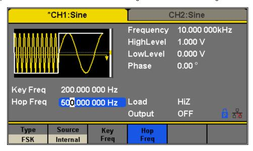
Figure 80 - Generate a FSK Modulation Waveform
