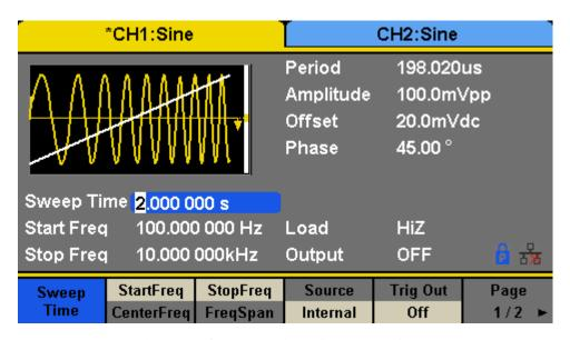
Figure 75 - Generate a Linear Sweep Waveform
