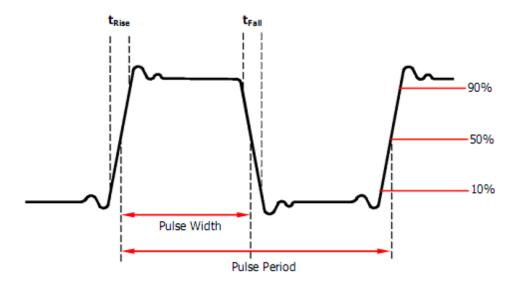
Figure 12 - Pulse Width and Period
