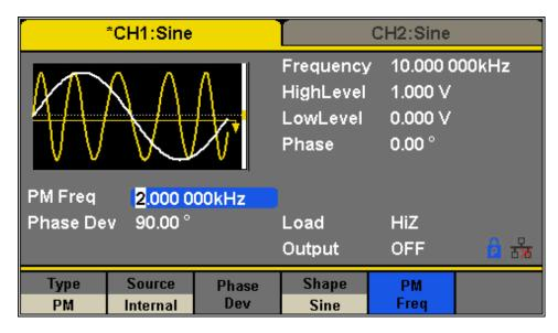
Figure 79 - Generate a PM Modulation Waveform
