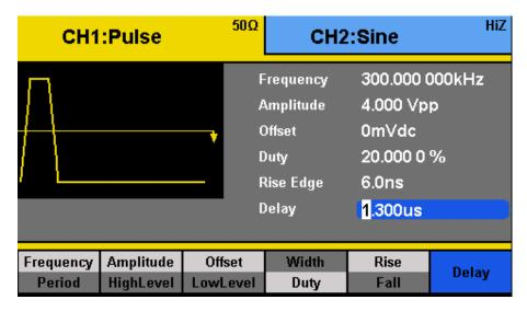
Figure 16 - Pulse Delay
