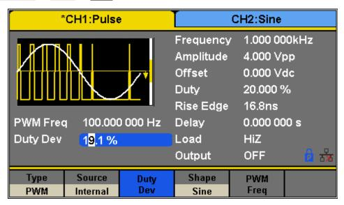
Figure 35 - Setting Interface of PWM Modulation
