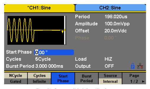
Figure 76 - Generate a N-Cycle Burst Waveform
