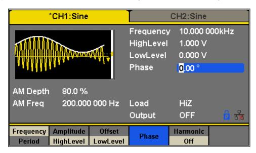
Figure 77 - Generate an AM Modulation Waveform
