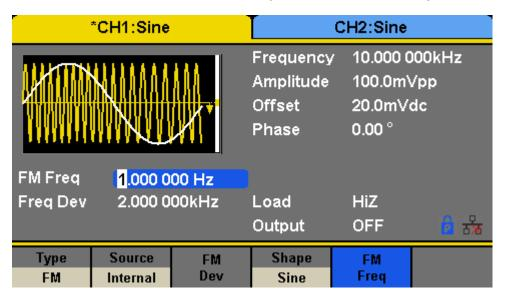
Figure 78 - Generate a FM Modulation Waveform
