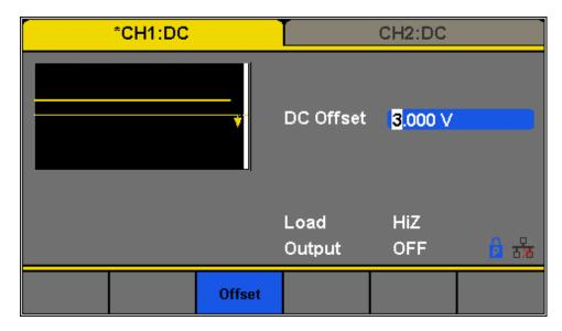
Figure 74 - Generate a DC Waveform
