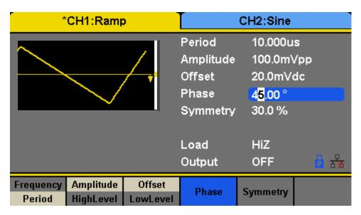
Figure 71 - Generate a Ramp Waveform
