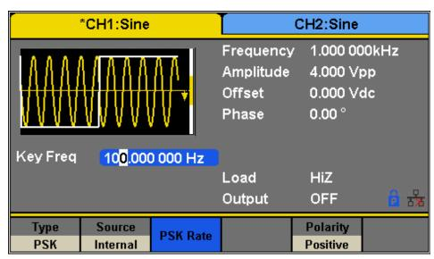
Figure 34 - Setting Interface of PSK Modulation
