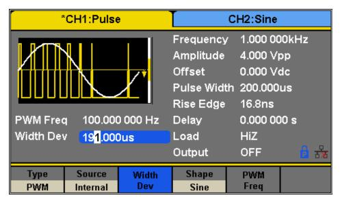
Figure 36 - Width Deviation Setting Interface
