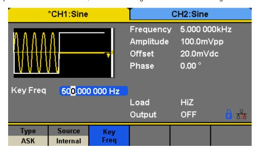
Figure 81 - Generate a ASK Modulation Waveform
