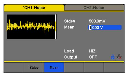
Figure 73 - Generate a Noise Waveform
