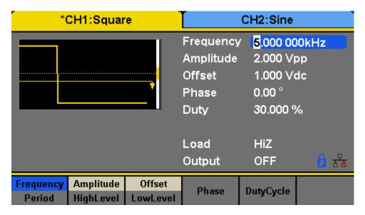
Figure 70 - Generate a Square Waveform
