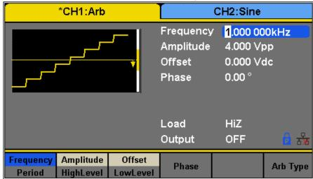
Figure 24 - Configuring an Arbitrary Waveform
