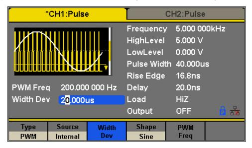
Figure 83 - Generate a PWM Waveform
