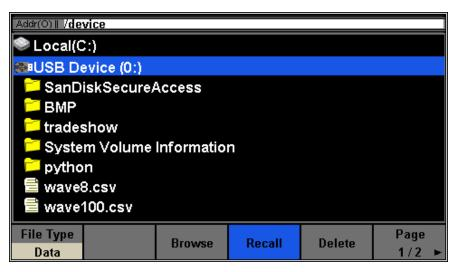
Figure 26- Load an Arb Waveform from External USB
