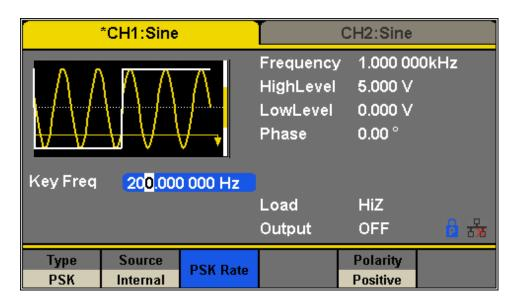
Figure 82 - Generate a PSK Modulation Waveform
