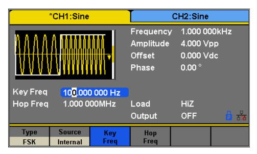
Figure 32 - Setting Interface of FSK Modulation
