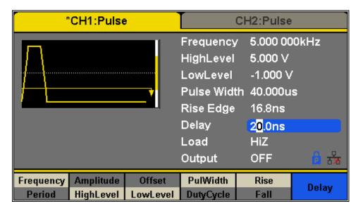
Figure 72 - Generate a Pulse Waveform
