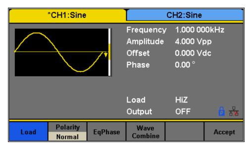
Figure 57 - Output Setup
