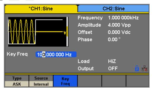
Figure 33 - Setting Interface of ASK Modulation
