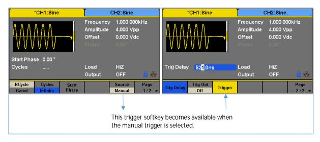
Figure 43 - NCycle Burst Manual Trigger
