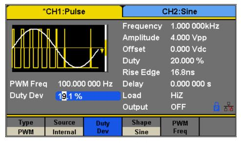
Figure 37 - Duty Deviation Setting Interface
