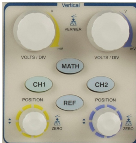
Figure 14 - Vertical System Controls
