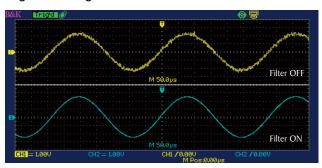
Filter out unwanted signal components such as various types of noise with built-in digital filters. Choose from Low-Pass, High-Pass, Band-Pass, and Band-Stop filters.
