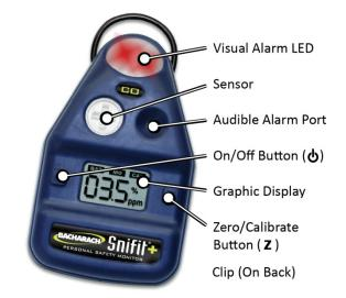
**Mounting:** The instrument may be attached using the metal lanyard loop or the sturdy suspender clip on the back of the instrument.
