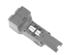
**Step 1** To gain access to the battery compartment, remove the bottom end of the strap assembly by detaching the Velcro connection and pulling the bottom end of the strap from the retaining pin in the bottom of the case of the base unit.
