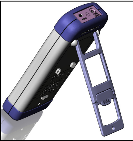
Folded up the bottom of the bracket to achieve degree 45 position Figure 1-3 Position of Degree 45
