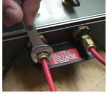
Connect clean, dry and oil-free air or nitrogen to the INLET valve. Connect instrument to be tested to the OUTLET valve.
