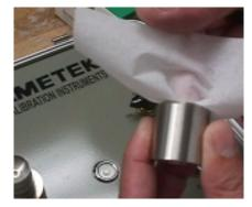
Using a cottom swab or soft cloth with a solvent such as alcohol, wipe the inside of the nozzle.
