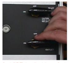
Open the OUTLET valve to calibrate the instrument. Once the calibration is completed, you may vent the pressure by rotating the OUTLET knob to the VENT position.
