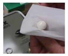
Dampen a clean cloth with alcohol or other residue-resistant solvent, and clean the ceramic ball by rotating it within the cloth.
