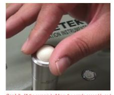
Carefully, lift the ceramic ball from the nozzle assembly and store in a secure location.
