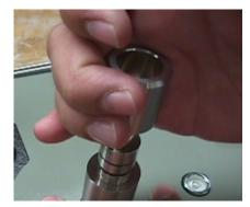
Grasp the nozzle firmly and pull upward with a slight twisting motion.
