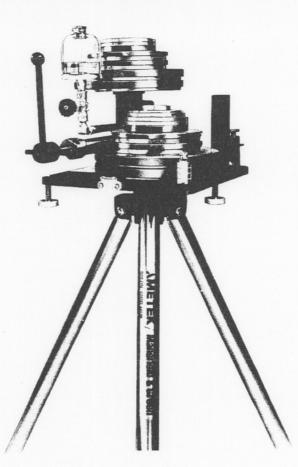
VIEW SHOWING HYDRA-LITE DEADWEIGHT TESTER MOUNTED ON OPTIONAL TRIPOD.
