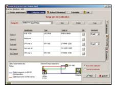
JOFRACAL calibration software may also be used for manual calibrations, as it can be set up to accept manual entry of calibration data together with other liquid baths, ice points or dry-block heat sources.
